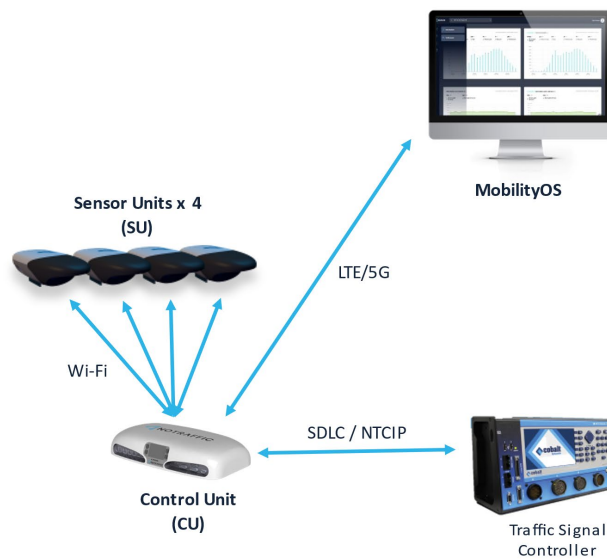
Figure 1: NoTraffic system Overview
